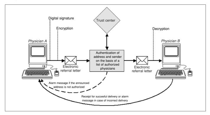
Figure 2. 'PaDok®'-communication network for the secure exchange of data
